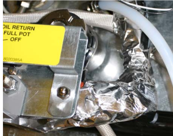
Figure 8: Cover heat tape with aluminum insulating tape.
