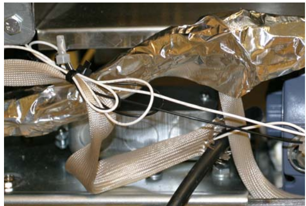
Figure 5: Secure wires securely with ty wraps.
