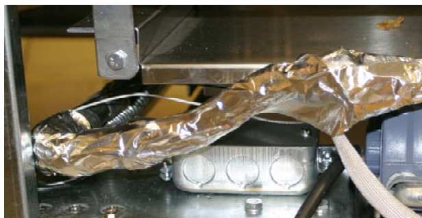
Figure 3: Secure the heater tape with insulating aluminum tape.
